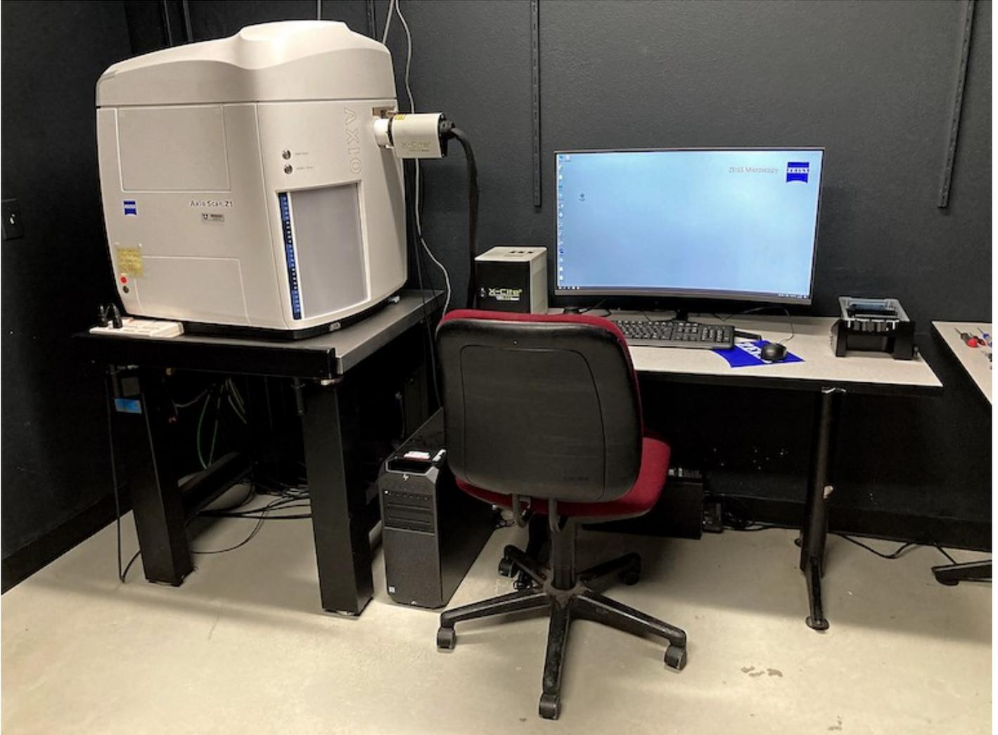
The Zeiss Axio-Scan.Z1 is a fast and flexible slide scanner that digitizes specimens to produce high-quality virtual slides. In addition to brightfield slide scanning, the Axio-Scan.Z1 uses LED lights to scan up to nine fluorescent channels. Up to 100 slides can be loaded onto the scanner, making it suitable for large projects, including digital archives. Scanned images are saved as CZI files and can be viewed using Zeiss freeware Zen-lite or third-party image analysis programs.
