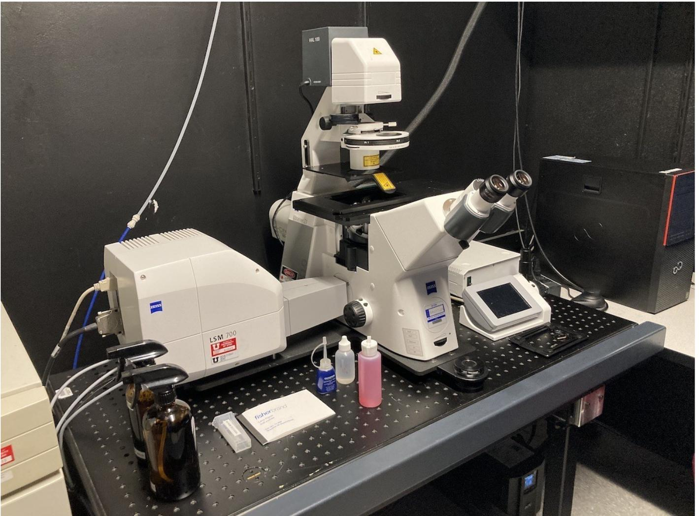
The LSM 700 laser scanning confocal microscope is the seventh generation of confocal microscopes from Carl Zeiss. The LSM 700 system uses a Zeiss AXIO Observer Z1 inverted microscope with transmitted illumination (HAL 100) and a laser illumination source. The LSM 700 system features easy operation, excellent sensitivity, and a design that can handle complex tasks.
