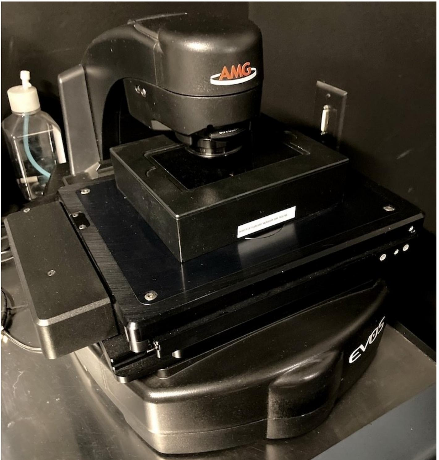
The EVOS FL Imaging system is an all-in-one fluorescence microscope designed for efficiency and ease of use. The on-board computer and integrated imaging software allows users to capture and save four channels fluorescence images/data directly from the microscope. The EVOS FL Imaging System is suitable for checking samples before using a high-end microscope system.
