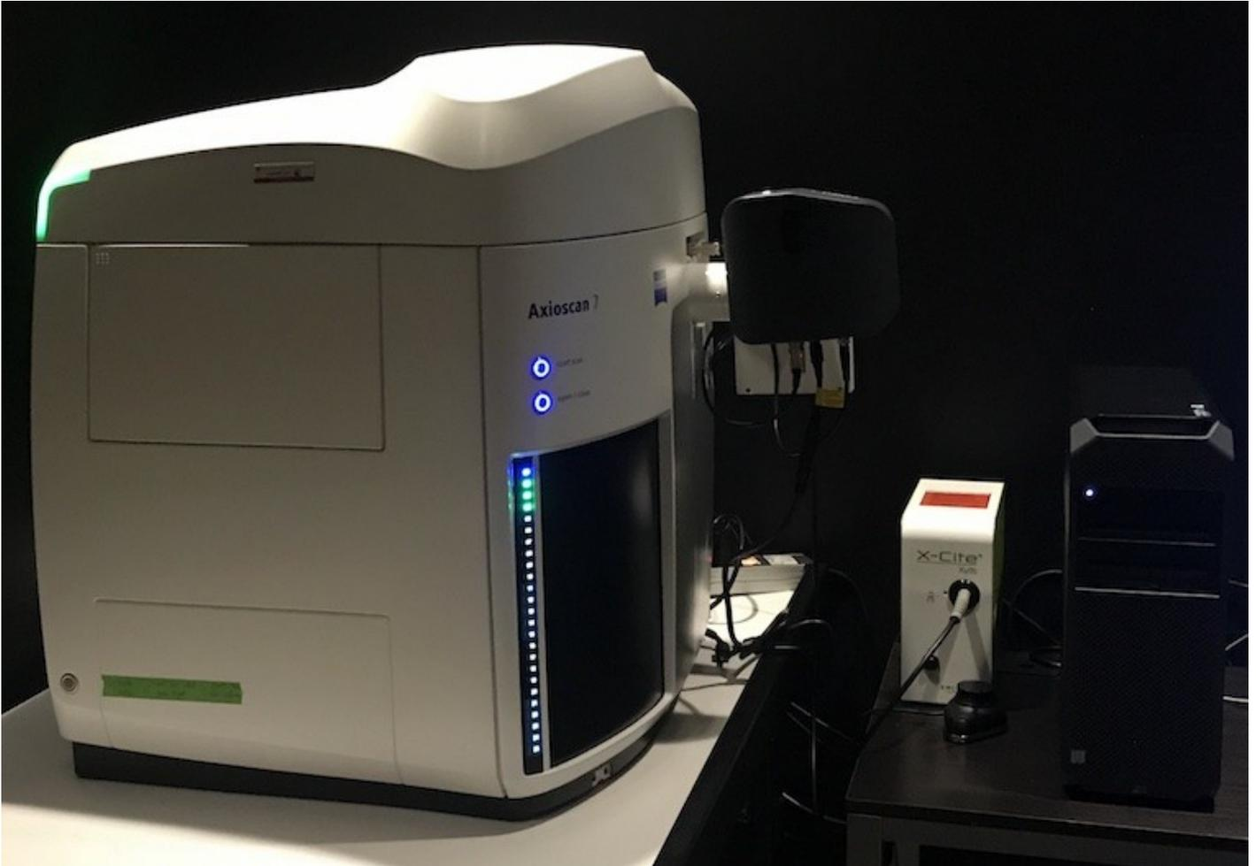
The Zeiss AxioScan 7 is a fast and flexible slide scanner that digitizes specimens to produce high-quality virtual slides. In addition to brightfield slide scanning, the Axioscan 7 can scan up to five fluorescent channels using fast switching LED lights. Up to 100 slides can be loaded onto the scanner, making it suitable for large projects, including digital archives. Scanned images are saved as CZI files and can be viewed using Zeiss freeware Zen-lite or third-party image analysis programs.
