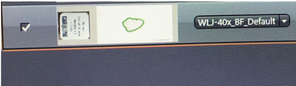
If some need a different profile, they can be set on a slide by slide basis in the Magazine view. The down arrow by the slides profile will show a list of all of the scan profiles you can select.
