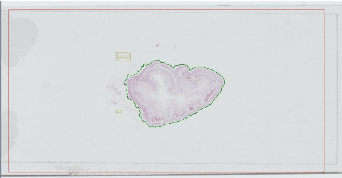
In the center of the screen will be the results of any automatic tissue detection. The green shapes are the detected tissues. If there are tan areas, they are areas that are used for collecting shading correction data. A red rectangle is the area of the slide that was used for tissue detection.
