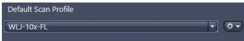
There is always a default scan profile. If you are going to adapt a profile, select the default profile from the drop down list. If you want to start from scratch, use the gear tool to start a new profile.
